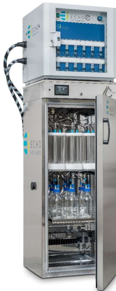
Figure 3: 12-channel respirometer for automatic biodegradation measurements
